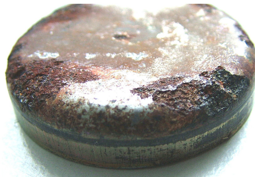
A 6 Sealing cover, corroded
