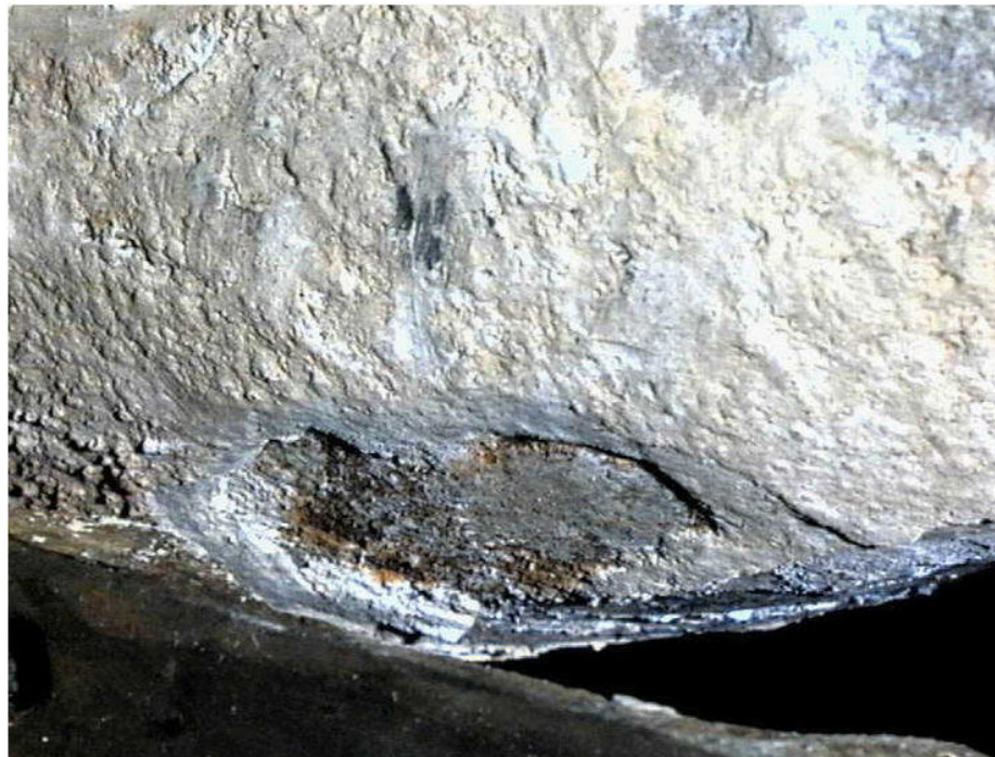
A 8 Limescale deposits on a cylinder liner
