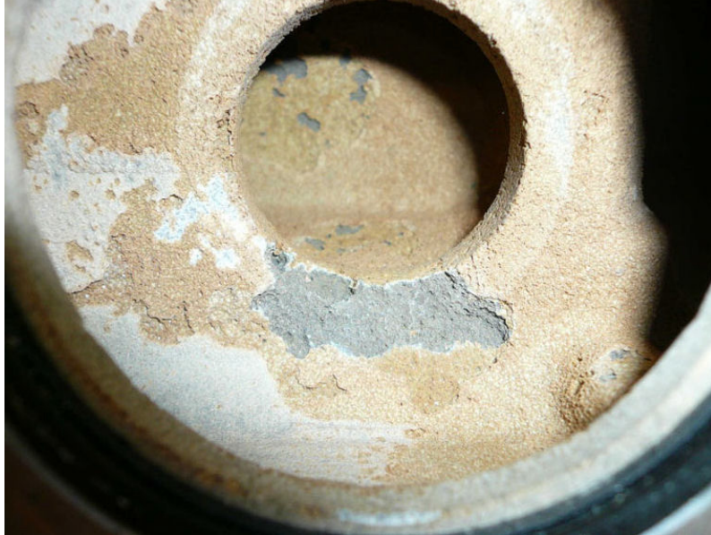
A 7 Aluminium thermostat cover, corroded
